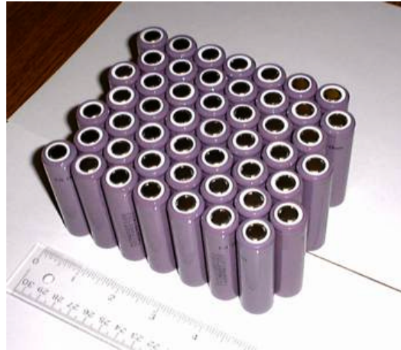
Sample EV sized module - 100Ah
